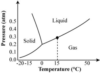
The temperature of the substance is 15°C. At what pressure would the liquid phase of the substance changes to its vapor state?
